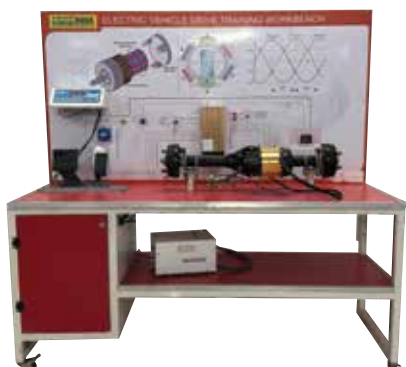
Electric Vehicle Drivetrain with Variable Load Monitoring System
