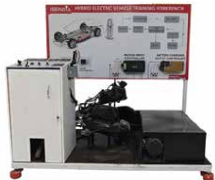
Hybrid Vehicle Training setup enabled with Data Acquisition System
