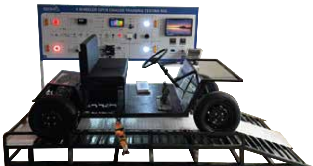
4 Wheeler EV Powertrain for Performance Analysis using Open ECU with Road Behaviour Simulations
