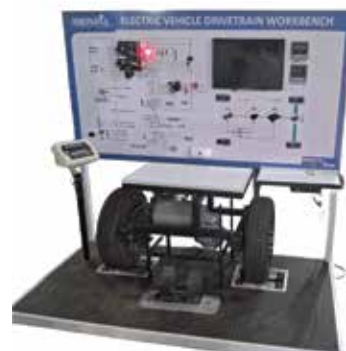
AI-Enabled EV Drivetrain for Performance Analysis using Open ECU
