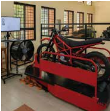
Electric 2-W Chassis Dyno with Variable Load Simulation and Diagnosis
