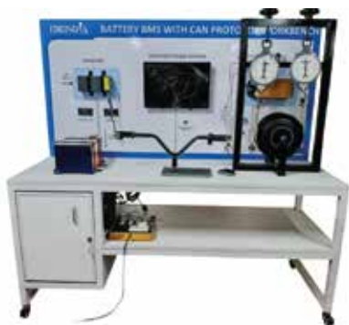
AI - Enabled BMS Test bench with Varying parameters for Performance analysis and Algo design using CAN Protocol
