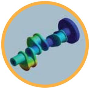
Fatigue Analysis - Crank Shaft
