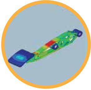
Linear Static Analysis - Brake Pedal
