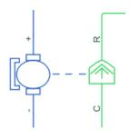
Define the parameter Rated Voltage= 320V Rated Load = 84 kW No-Load Speed = 10000 rpm Rated Speed = 3796 rpm
