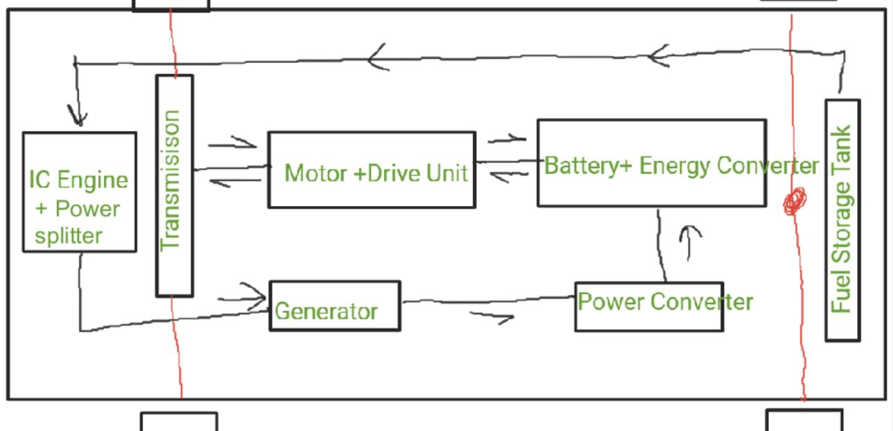
This is modification to series type, here power splitter is used to divide power between the transmission and generator. At the same time battery can be charged and also the power can be transferred via transmission system.
