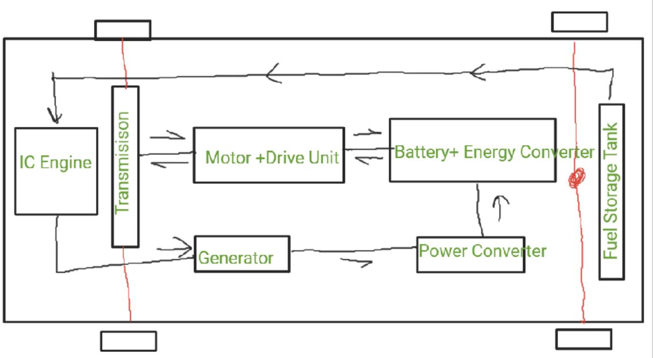
In this system the unlike Parralel type, the IC engine here is connected to a generator instead of transmission system. This generator charges battery and in return the Motor drives the transmission system. Here battery is the major soruce of power transmission
