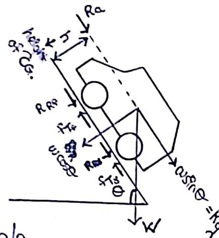
Q.1. Derive the equation of motion and maximum tractive effort for a car inclined at angle  $\theta$ . Also give the expression of maximum gradeability for a 4 wheel drive. (cont.)
