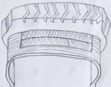
Radial tyres are constructed with rubber coated reinforcing steel cable belts that are assembled parallel and run from side to side, bead to bead at an angle of 90 degrees to the circumferential centre line of the tyre.
