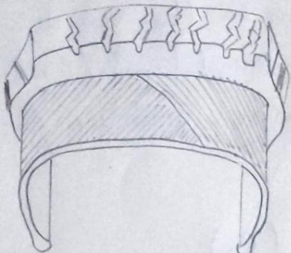
Bias ply construction utilises rubber layers called plies that are placed diagonally from one bead to another bead at an angle not exceeding 30 degrees to each other.
