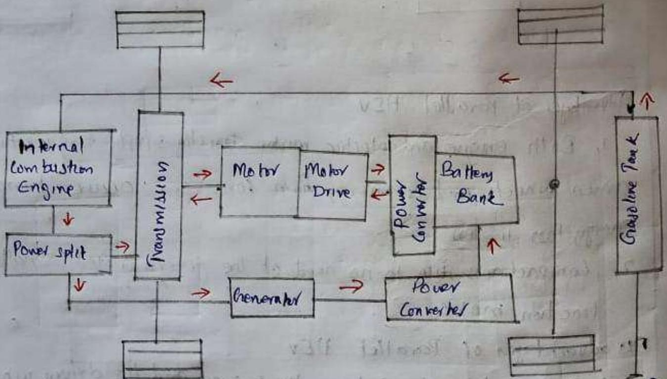
\* The Series Parallel Hybrid vehicle have feature of both Series and Parallel hybrid \* Many different modes of driving are possible under IC engine dominant Hybrid
