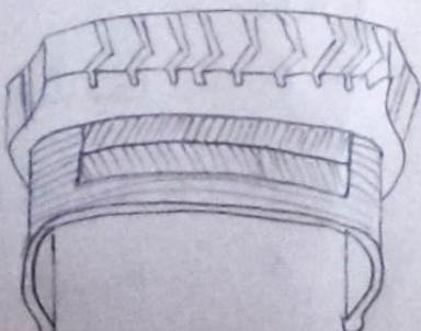
Radial tyres are constructed with rubber coated, reinforcing steel cable belts that are assembled parallel and run from side to side, bead to bead at an angle of 90 degrees to the circumferential centre line of the tire.
