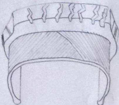
Bias ply construction utilises rubber layers called plies that are placed diagonally from one bead to another bead at an angle not exceeding 30 degrees to each other.
