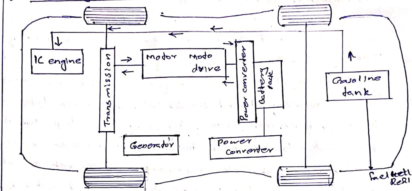
series hybrid EV which IC engine is not directly connected to transmission. The IC engine which may directly connected to Generators and also power converter which may help to charge the battery part and which battery may connected to motor or motor will drive the vehicle to transmission. This made vehicle drive.
