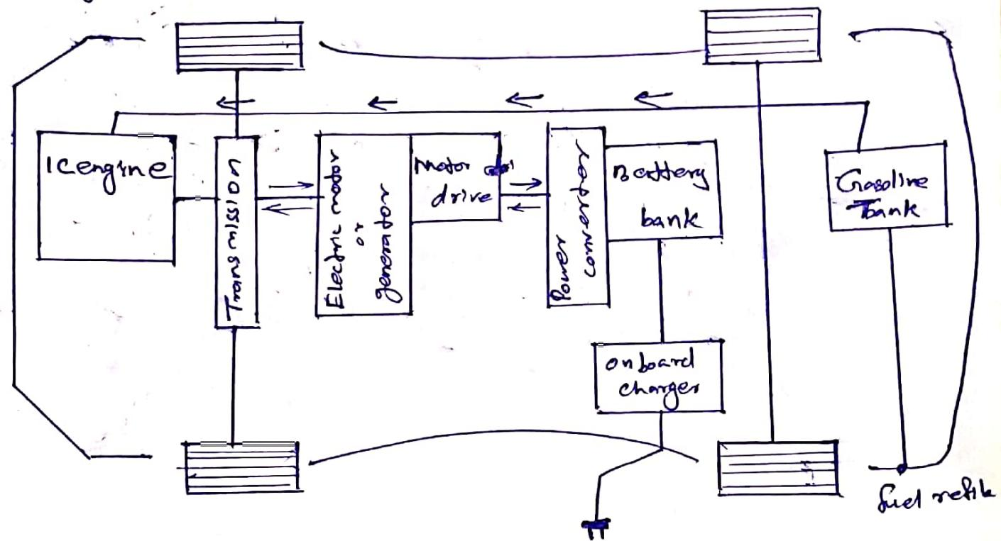
In plug in hybrid the function is same as 'the hybrid' but the only change is there is an onboard charger plug is for charging. other working working as same there is a plug to recharge the battery pack.
