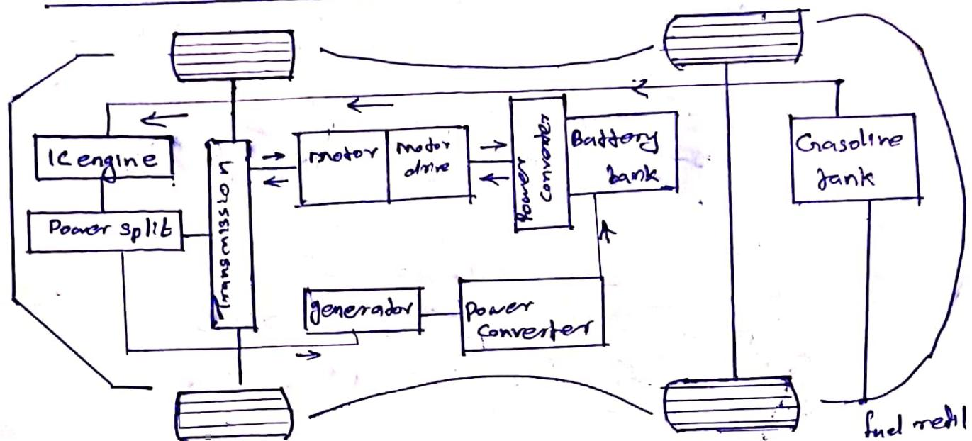
In this motor is directly connected to the transmission.
