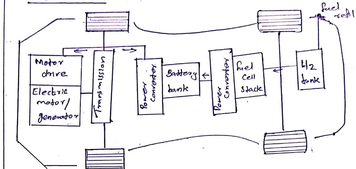
In fuel cell eEV there is no IC engine is used. Here instead we use fuel cells that generate electricity. ~~However to~~ we have to refill it at hydrogen charging station. In this the power is generated by the reaction with oxygen and water and heat is produced as byproduct.
