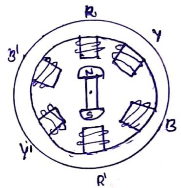
Working Principle :- The BLDC motor works on the Lorenze force principle. It state that when ever a current carrying conductor placed in a magnetic field it experience - equal & opposite force or torque. The direction of motion varies continuously with time in BLDC. This variation is due to the voltage by current.
