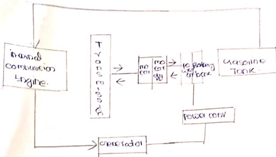
\* Series hybrid electric vehicle is an electric vehicle which assisted by an internal combustion engine and Transmission system does not have direct connection with internal combustion engine.
