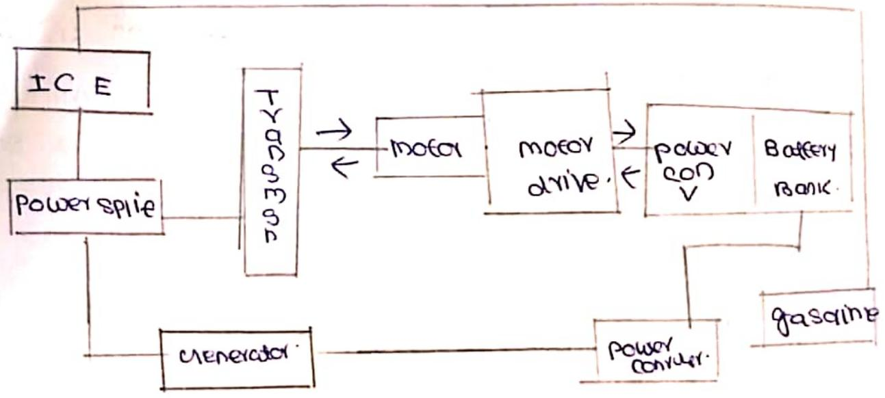
\* Here a power split is used to connect ICE with E-transmission and generator at same time and have features of both series and parallel hybrid Toyota prius is the first model.
