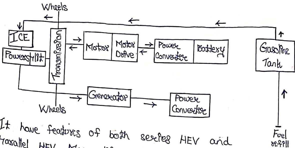
It has features of both series HEV and parallel HEV. Many different modes of driving is possible under ICE dominant hybrid vehicle and under motor dominant drive mode. The first model used in a vehicle was on the Toyota Prius on 1997. The drawback of the series was that it was very bulky.
