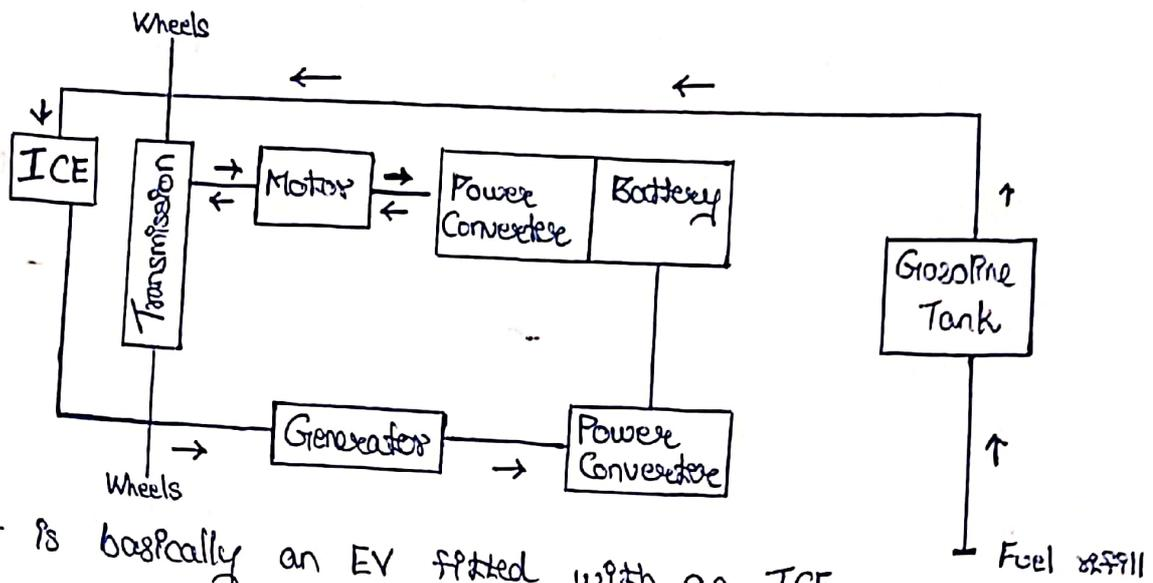
It is basically an EV fitted with an ICE to recharge the battery pack. Here the motor is the primary source, and hence more powerful than the ICE. Hence the battery pack will be large in size.
