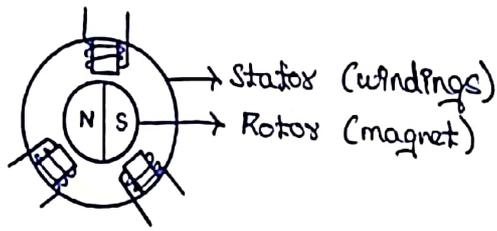
The BLDC motor uses a permanent magnet as the rotor. The coils that carry the current are fixed on the stator. When you pass current through the # coils, the resultant magnetic current attracts or deflects the permanent magnet, which in the case is the rotor itself. By adjusting the magnitude and direction of the current into the coils using a controller, the direction and speed of the rotor's rotation can be controlled (unlike the brushed DC motor which uses brushes and commutator).
