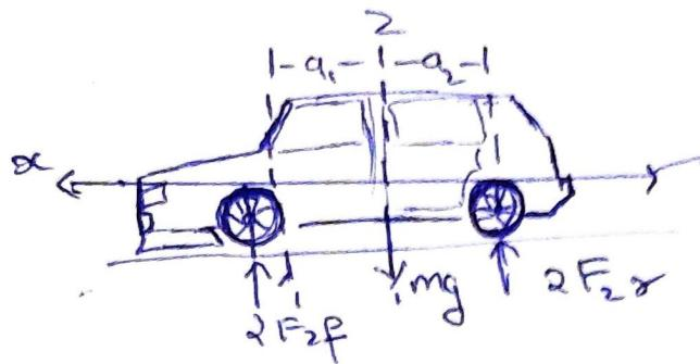
when car parked on level road . The normal force i.e. ( $F_z$ ) under each of front & rear wheel ( $F_{zf}$ ) ( $F_{zr}$ ) are.
