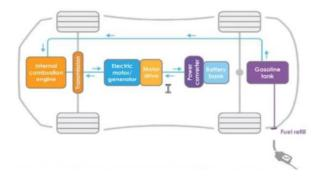
In vehicles with parallel hybrid drivetrains, the engine and electric motor work in tandem to generate the power that drives the wheels. Parallel hybrids tend to use a smaller battery pack than series drivetrains, relying on regenerative braking to keep it recharged. When power demands are low, parallel hybrids also utilize the motor as a generator for supplemental recharging, much like an alternator in conventional cars.
