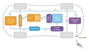
Series drivetrains are the simplest hybrid configuration. In a series hybrid, the electric motor is the only means of providing power to the wheels. The motor receives electric power from either the battery pack or from a generator run by a gasoline engine. A computer determines how much of the power comes from the battery or the engine/generator. Both the engine/generator and the use of regenerative braking recharge the battery pack.
