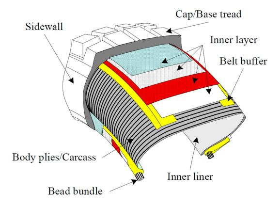
A tire is an advanced engineering product made of rubber and a series of synthetic materials cooked together. Fiber, textile, and steel cords are some of the components that go into the tire's inner liner, body plies, bead bundle, belts, sidewalls, and tread. Bead or bead bundle is a loop of high strength steel cable coated with rubber. It gives the tire the strength it needs to stay seated on the wheel rim and to transfer the tire forces to the rim.
