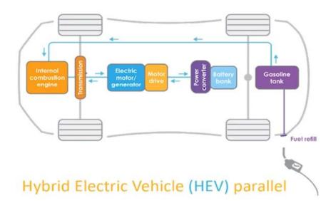
In Parallel hybrid Vehicle IC engine is the primary source , Electric motor is secondary source
