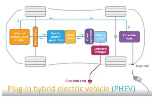
Plug in Hybrid electric vehicle ICE is the More powerful than electric motor
