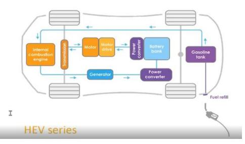
In series hybrid Vehicle electric Motor is the primary source , IC engine is secondary source
